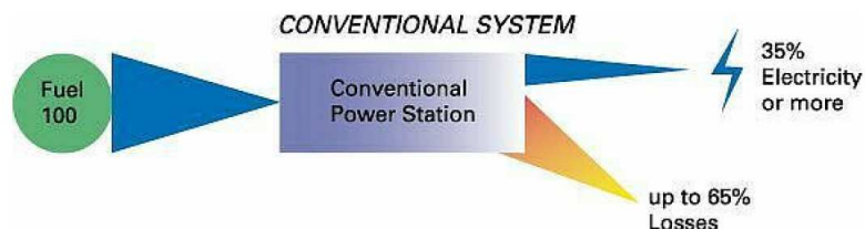
Figure 8: Typical conventional power generation scheme. Source: Unep, 2009
